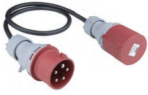
Cable: H07RN-F 5 x 2.5mmsq, or PVC 4C x 14AWG Connector: 32A 3P+N+E CEE form (380V)
