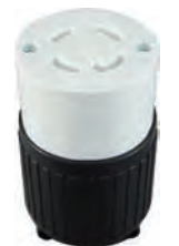
ATL-1430C Locking Cord Connector Pin: 4 / AMP: 30 / Voltage: 125 / 250 NEMA: L14-30P
