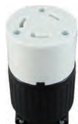
ATL-630C Locking Cord Connector Pin: 3 / AMP: 30 / Voltage: 250 NEMA: L6-30C
