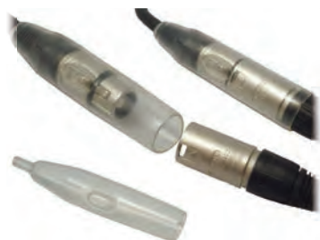
XLR-WPC XLR Water Proof Cover XLR-WPC is designed to protect XLR connector from wet and dust. See-through transparent PVC body helps check up mating status easily. Feasible for O.D. 4-6 mm cable. IP66.
