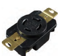
ATL-1420R Locking Receptacle Pin: 4 / AMP: 20 / Voltage: 125 / 250 NEMA: L14-20R
