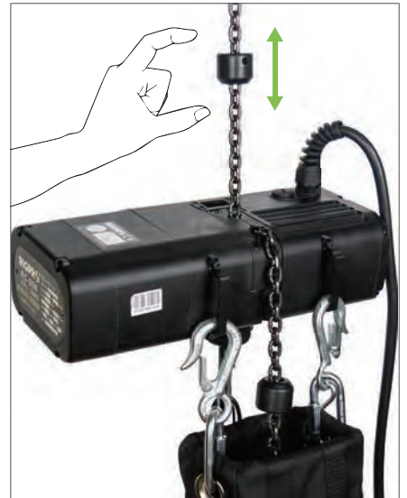
Slide the positioning block along the chain to set up the hoist travel limit. Opening side cap to adjust is not required. Absolutely tool free.
