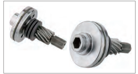
Friction clutch with lining is located outside the load patch so that the load is firmly held by brakes while hoist is disconnected from power
