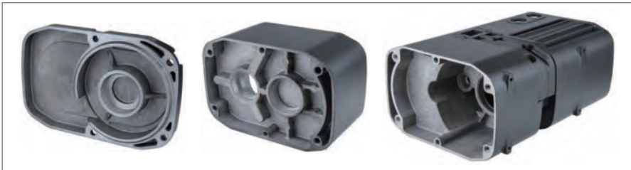
Die-casting aluminum housing for the greatest toughness and robustness, yet lightweight. Black epoxy powder finish for less visibility and corrosion resistance. Rated for IP65 with housing completely assembled and treatment.
